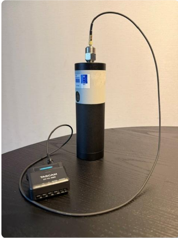
Calibrated Vibration Signal 10 mm/s rms & 159.2 Hz
